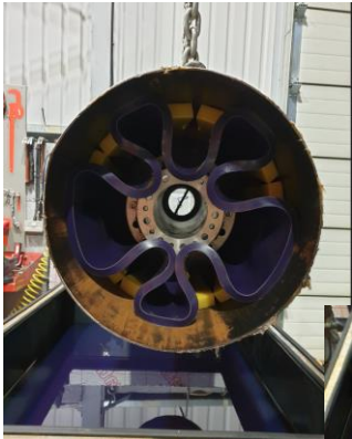
Dual diameter pig undergoing heat trials in diesel at 50 °c whilst in a compressed state
