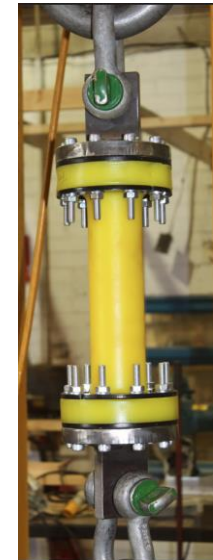
Dual diameter pig tow arm pull test
